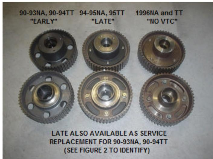
Figure 1 – VG30DE(TT) Intake Pulley Identification
